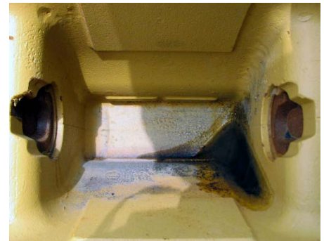
Hensley and CAT point cavities without proper contour for stabilization.
