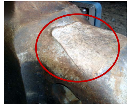
S-Series Posilok nose with severe wear and deformation caused by using a Hensley adapter
