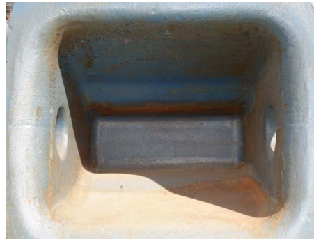
Hensley and CAT point cavities without proper contour for stabilization.
