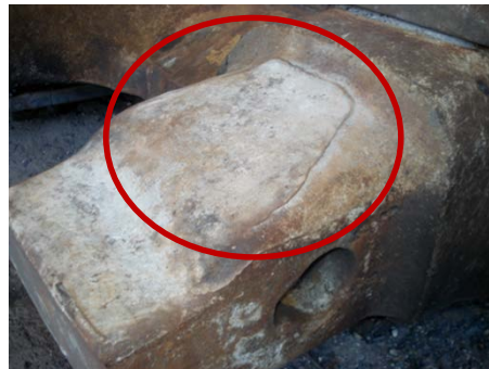
S-Series Posilok nose with severe wear and deformation caused by using a Hensley adapter
