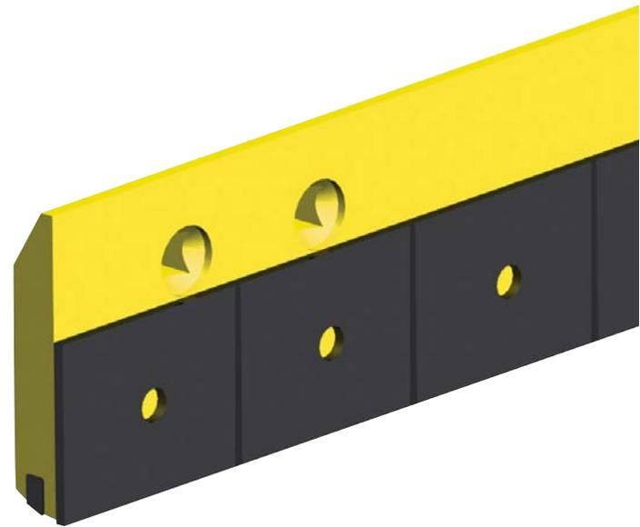
Kennametal Armored Blades are designed to provide better protection of the steel face of standard carbide insert blades. When working on unpaved surfaces, the mild steel can deteriorate, exposing the carbide insert to greater impact and causing blade breakage. Kennametal Armored Blades are the economical choice to prevent this type of wear.
